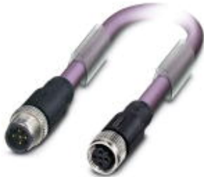
Bus system cable, PROFIBUS, PROFIBUS, 2-position, PUR halogen-free, Violet, RAL 4001, shielded, Plug straight M12, B-coded, on Socket straight M12, B-coded, Cable length: 10 m
