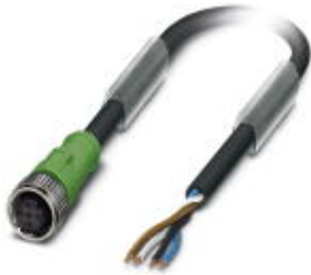
Sensor/Actuator cable, 4-position, PUR, Black-gray RAL 7021, Free cable end, on Socket straight M12, A-coded, Cable length: 10 m
