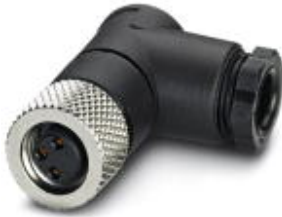
Sensor/actuator connector, female, angled, 4-pos., M8, solder connection, metal knurl, cable diameter max. 5 mm
