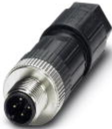
Connector, 4-position, Plug straight M12, A-coded, Spring-cage conn., Knurl material: Zinc die-cast, nickel-plated, External cable diameter 4 mm ... 8 mm
