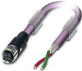
Bus system cable, PROFIBUS, PROFIBUS, 2-position, PUR halogen-free, Violet, RAL 4001, shielded, Free cable end, on Socket straight M12 SPEEDCON, B-coded, Cable length: 2 m
