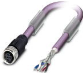
Bus system cable, CANopen ® , DeviceNet ™ , CANopen ® /DeviceNet ™ , 5-position, PUR halogen-free, Violet, RAL 4001, shielded, Free cable end, on Socket angled M12, A-coded, Cable length: 0.5 m
