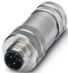
Bus system connector, male, straight, 4-pos., M12, shielded, D-coded, screw connection, metal knurl, cable screw connection Pg7
