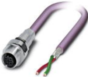
Bus system flush-type socket, PROFIBUS, 2-pos., M12, shielded, B-coded, front/screw mounting with M16 thread, with 0.5 m bus cable, 2 x 0.25 mm 2
