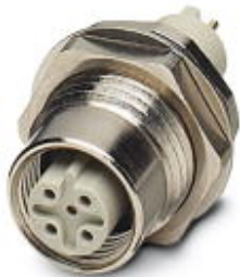
Sensor/Actuator flush-type socket, 5-pos., M12, B-coded, rear/screw mounting with Pg9 thread, with straight solder connection
