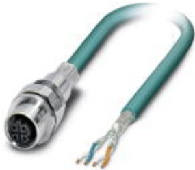
Bus system flush-type socket, ETHERNET, 4-pos., M12, shielded, D-coded, front/screw mounting with M16 thread, can be positioned, with 1 m bus cable, 2 x 2 x 0.14 mm 2
