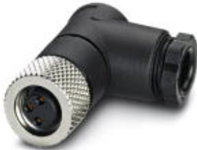
Sensor/actuator connector, female, angled, 3-pos., M8, solder connection, metal knurl, cable diameter max. 5 mm
