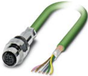
Bus system flush-type socket, INTERBUS, 5-pos., M12, shielded, B-coded, front/screw mounting with M16 thread, can be positioned, with 0.5 m bus cable, 3 x 2 x 0.25 mm 2
