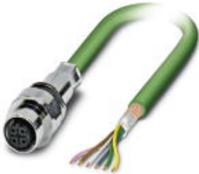
Bus system flush-type socket, INTERBUS, 5-pos., M12, shielded, B-coded, front/screw mounting with M16 thread, can be positioned, with 1 m bus cable, 3 x 2 x 0.25 mm 2
