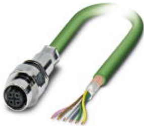
Bus system flush-type socket, INTERBUS, 5-pos., M12, shielded, B-coded, front/screw mounting with M16 thread, can be positioned, with 5 m bus cable, 3 x 2 x 0.25 mm 2
