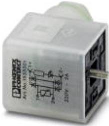
Valve connector, 3-pos., type A, 1 LED, with protective circuit and rectifier, screw connection, cable screw connection Pg9
