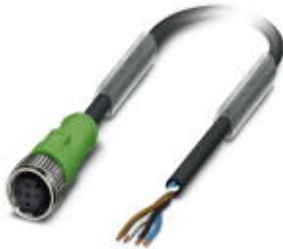
Sensor/Actuator cable, 4-position, PUR halogen-free, Black-gray RAL 7021, Free cable end, on Socket straight M12, A-coded, Cable length: 2 m
