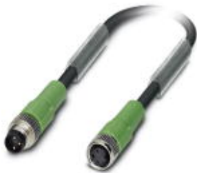
Sensor/Actuator cable, 3-position, PUR, Black-gray RAL 7021, Plug straight M8, A-coded, on Socket straight M8, A-coded, Cable length: 2.5 m
