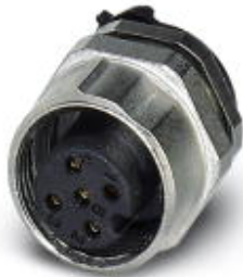
Sensor/actuator flush-type socket, 5-pos., M12 SPEEDCON, A-coded, rear/screw mounting with M12 thread, with polarity protection, with straight THR solder connection
