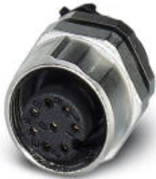
Sensor/actuator flush-type connector, socket, 8-pos., M12 SPEEDCON, A-coded, rear/screw mounting with M12 thread, with polarity protection, with straight THR solder connection
