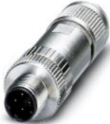
Bus system connector, Ethernet CAT5, Ethernet CAT5e, 4-position, shielded, Plug straight M12, D-coded, Insulation displacement connection, Knurl material: Nickel-plated brass, External cable diameter 4 mm ... 8 mm
