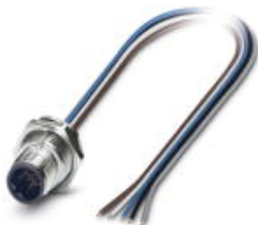
Sensor/actuator flush-type connector, 5-pos., M12 SPEEDCON, B-coded, rear/screw mounting with Pg9 thread, with 0.5 m TPE litz wire, 5 x 0.34 mm²
