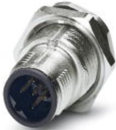
Sensor/actuator flush-type plug, 5-pos., M12-SPEEDCON, B-coded, rear/screw mounting with Pg9 thread, with straight solder connection, design with 12 mm long solder pins
