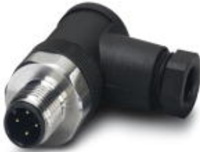
Sensor/actuator connector, male, angled, 4-pos., M12, screw connection, high-grade steel knurl, cable screw connection Pg7
