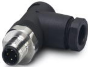
Sensor/actuator connector, male, angled, 4-pos., M12, screw connection, high-grade steel knurl, cable screw connection Pg9
