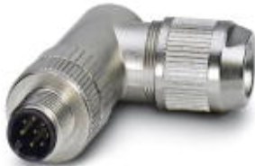
Bus system connector, Ethernet CAT5, Ethernet CAT5e, 8-position, shielded, Plug angled M12, A-coded, Insulation displacement connection, Knurl material: Nickel-plated brass, External cable diameter 4 mm ... 8 mm
