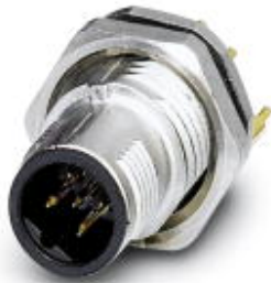
Sensor/actuator flush-type plug, 5-pos., M12 SPEEDCON, shielded, B-coded, rear/screw mounting with Pg9 thread, with straight solder connection, design with 12 mm long solder pins
