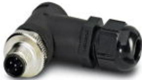
Sensor/actuator connector, angled, 5-pos., M12, A-coded, screw connection, metal knurl, SKINTOP® Pg9 cable gland
