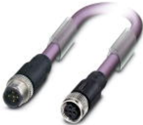
Bus system cable, PROFIBUS, PROFIBUS, 2-position, PUR halogen-free, Violet, RAL 4001, shielded, Plug straight M12, B-coded, on Socket straight M12, B-coded, Cable length: 12 m
