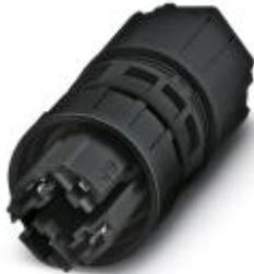
QUICKON connector, black, 4-pos. with PE, 1.0 mm 2 ... 2.5 mm 2 /630 V/20 A, for cables with a diameter of 9 mm ... 14 mm.
