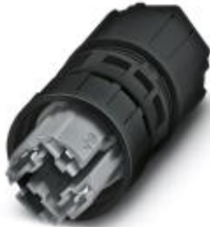
QUICKON connector, gray, 4-pos. without PE, 1.0 mm 2 ... 2.5 mm 2 /630 V/20 A, for cables with a diameter of 6 mm ... 10 mm.
