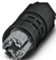
QUICKON connector, gray, 4-pos. without PE, 1.0 mm² ... 2.5 mm²/630 V/20 A, for cables with a diameter of 9 mm ... 14 mm.
