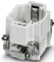
HEAVYCON male insert, DD24 series, 24-pos., crimp connection. PE connection using tension sleeve technology.
