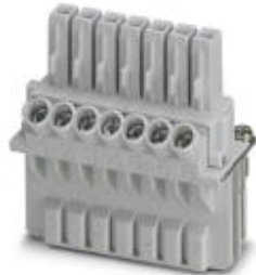
DUPLICON, connector contact insert, 6 x 4 mm 2 + PE, 400/690 V, 25 A, screw connection, type B6, IP20 protection
