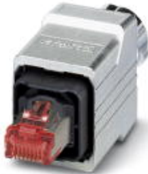
RJ45 connector, IP67, with push/pull interlocking (version 14), metal housing, for 1 Gbps, for 24 ... 25 AWG stranded conductors
