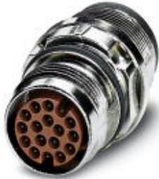
Device connector, front mounting, straight, SPEEDCON locking, M17, Number of positions: 17, Type of contact: Male connector, Crimp connection, Axial O-ring, Central fixing, shielded: Yes
