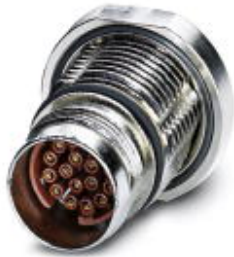
Device connector, rear mounting, straight, SPEEDCON locking, M17, Number of positions: 17, Type of contact: Socket, Crimp connection, Axial O-ring, Central fixing, shielded: Yes
