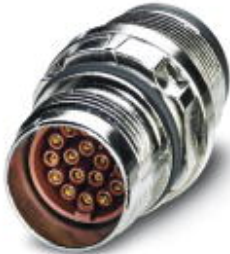
Device connector, front mounting, straight, SPEEDCON locking, M17, Number of positions: 8, Type of contact: Socket, Crimp connection, Axial O-ring, Central fixing, shielded: Yes
