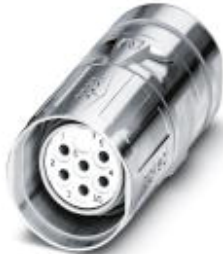
Cable connector, straight, shielded: Yes, SPEEDCON locking, M23, Number of positions: 7, Type of contact: Socket, Crimp connection, Cable diameter: 10 mm ... 14.5 mm
