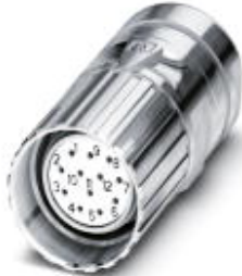
Cable connector, straight, shielded: Yes, Screw locking, M23, Number of positions: 17, Type of contact: Socket, Crimp connection, Cable diameter: 10 mm ... 14.5 mm
