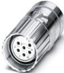
Cable connector, straight, shielded: Yes, Screw locking, M23, Number of positions: 7, Type of contact: Socket, Crimp connection, Cable diameter: 6 mm ... 10 mm
