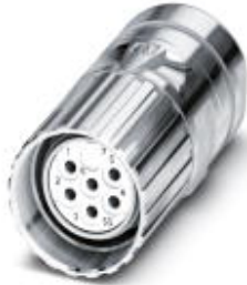
Cable connector, straight, shielded: Yes, Screw locking, M23, Number of positions: 7, Type of contact: Socket, Crimp connection, Cable diameter: 3 mm ... 14.5 mm
