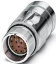
Coupling connector, straight, shielded: Yes, SPEEDCON locking, M23, Number of positions: 17, Type of contact: Socket, Crimp connection, Cable diameter: 10 mm ... 14.5 mm
