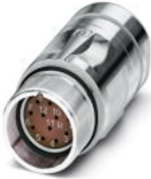
Coupling connector, straight, shielded: Yes, SPEEDCON locking, M23, Number of positions: 12, Type of contact: Socket, Crimp connection, Cable diameter: 10 mm ... 14.5 mm
