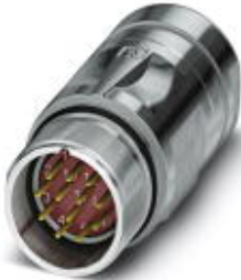
Coupling connector, straight, shielded: Yes, SPEEDCON locking, M23, Number of positions: 17, Type of contact: Male connector, Crimp connection, Cable diameter: 6 mm ... 10 mm
