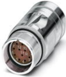
Coupling connector, straight, shielded: Yes, SPEEDCON locking, M23, Number of positions: 12, Type of contact: Socket, Crimp connection, Cable diameter: 3 mm ... 14.5 mm
