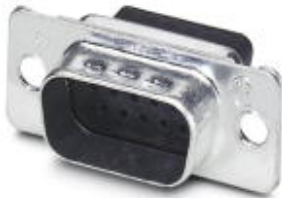
D-SUB contact carrier, shell size 1, for 15 signal contacts, contact type pin, for crimp contacts, straight, fixing with a 3 mm hole, for panel mounting frame and sleeve housing VS-09-...
