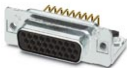
D-SUB contact insert, shell size 2, with 26 signal contacts, contact type socket, for PCB assembly, angled, fixing with 4-40 UNC thread and solder pins, for panel mounting frame VS-15-...
