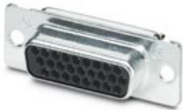
D-SUB contact insert, shell size 2, with 26 signal contacts, contact type socket, with solder cup, straight, fixing with a 3 mm hole, for panel mounting frame and sleeve housing VS-15-...
