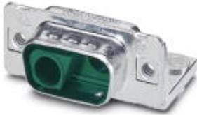
D-SUB contact carrier, shell size 1, accommodation for two combined contacts, contact type pin, fixing with 4-40 UNC thread and solder pins, for panel mounting frame VS-09-...
