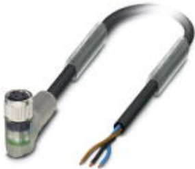
Sensor/Actuator cable, 3-position, PUR halogen-free, Black-gray RAL 7021, Free cable end, on Socket angled M8, with 2 LEDs, Cable length: 1.5 m
